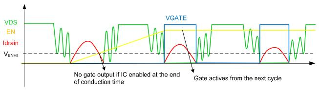
Figure 10: Synchronized Enable Function (resonant half-bridge)
