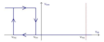
Figure 1: Input comparator thresholds
