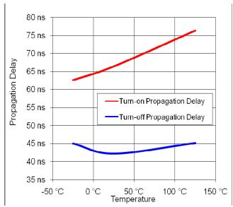
Figure 24: Turn-on and Turn-off Propagation Delay vs. Temperature
