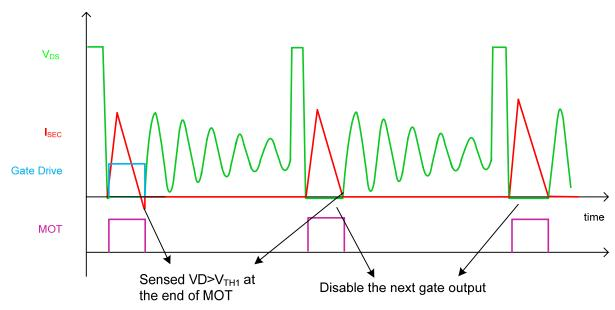
**Figure 9: MOT Protection Mode**
