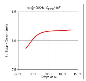
Figure 16: Icc Supply Currrent @1nF Load vs. Temperature
