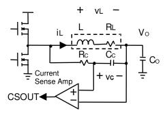
Figure 6 Inductor Current Sensing and Current Sense Amplifier
