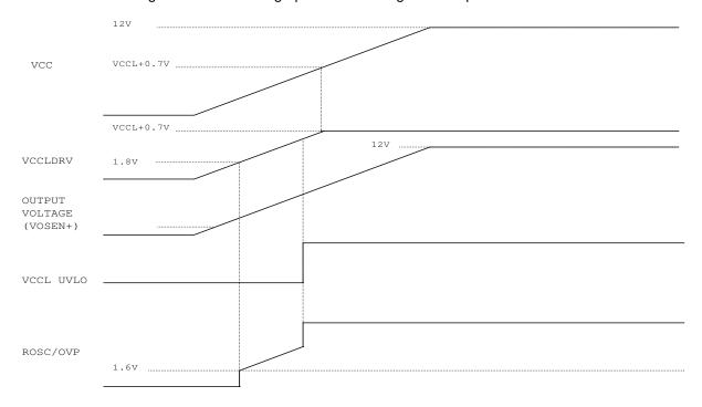
Figure 14 Over-voltage protection during power-up.
