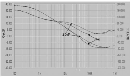
Figure 12 VCCL regulator stability with 5 phases and PHSOUT equals 750 kHz.
