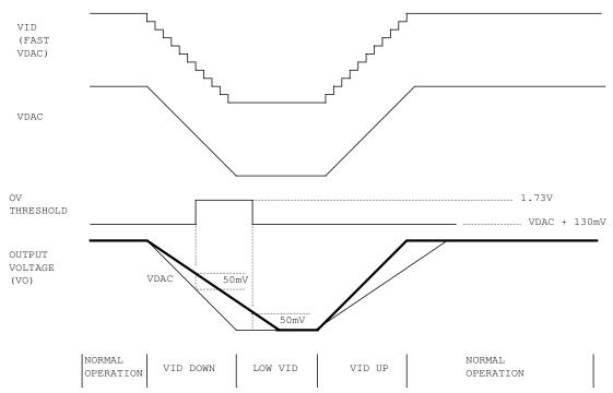
Figure 17 Over-voltage protection during dynamic VID
