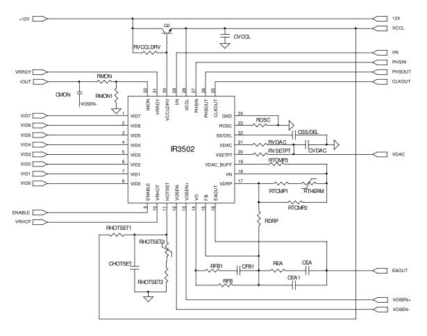
Figure 2 - IR3502 Application Circuit
