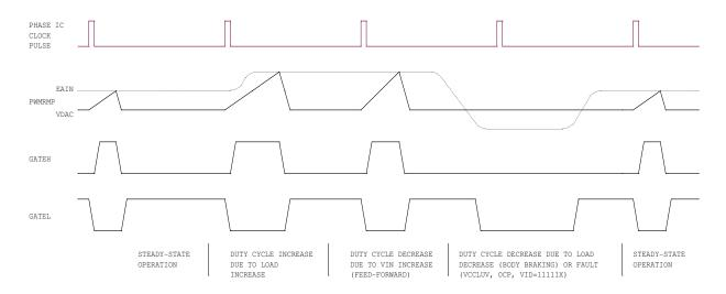
Figure 5 PWM Operating Waveforms
