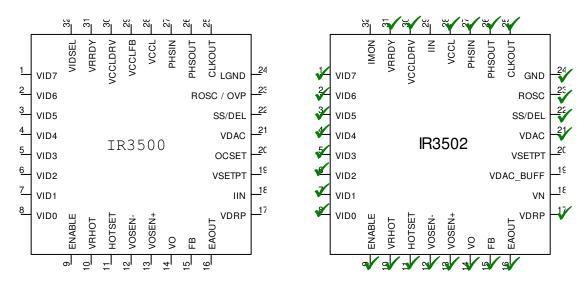
Figure 1 – PIN difference between IR3500 and IR3502
