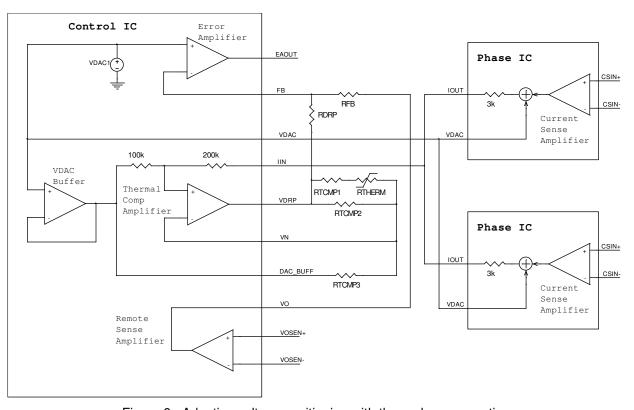
Figure 8 Adaptive voltage positioning with thermal compensation.
