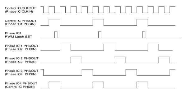
Figure 4 Four Phase Oscillator Waveforms
