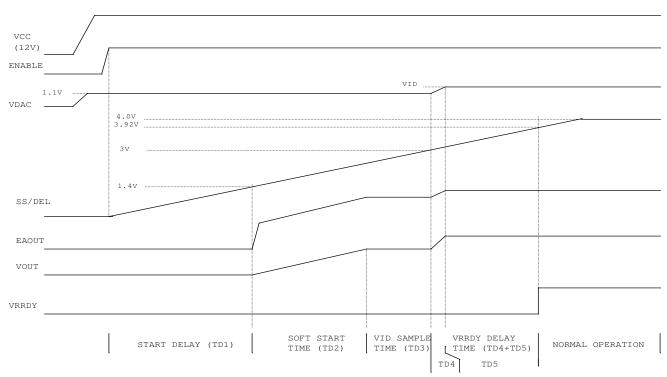
Figure 9 Start-up sequence of converter with boot voltage
