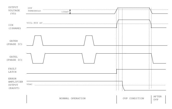
Figure 13 Over-voltage protection during normal operation
