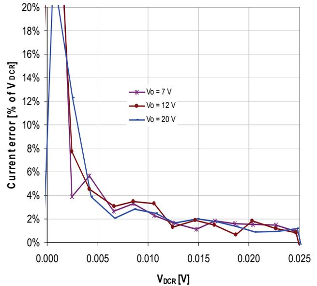
IR3725 CurrentMode - Error [%] (9 mV  $V_{DCR}$  full scale)
