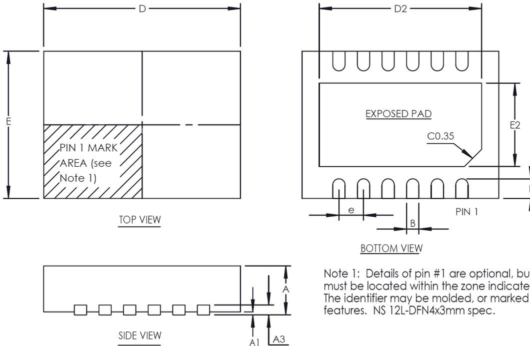
Note 1: Details of pin #1 are optional, but must be located within the zone indicated. The identifier may be molded, or marked features. NS 12L-DFN4x3mm spec.
