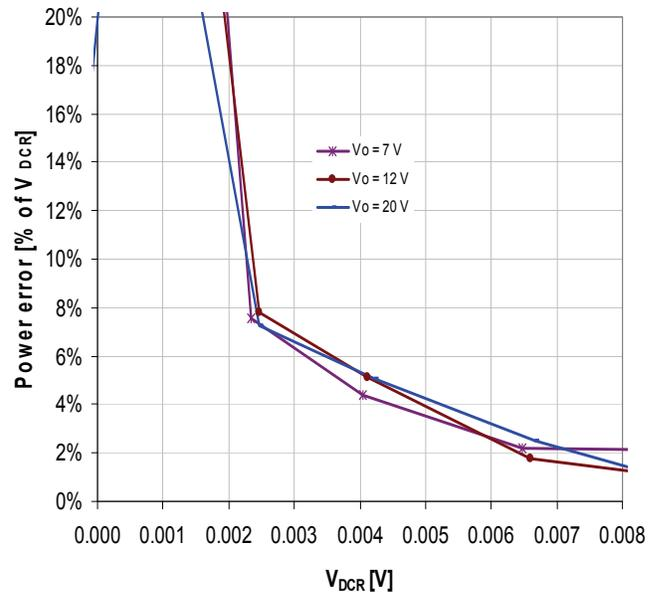
IR3725 CurrentMode - Error [%] (90 mV  $V_{DCR}$  full scale)
