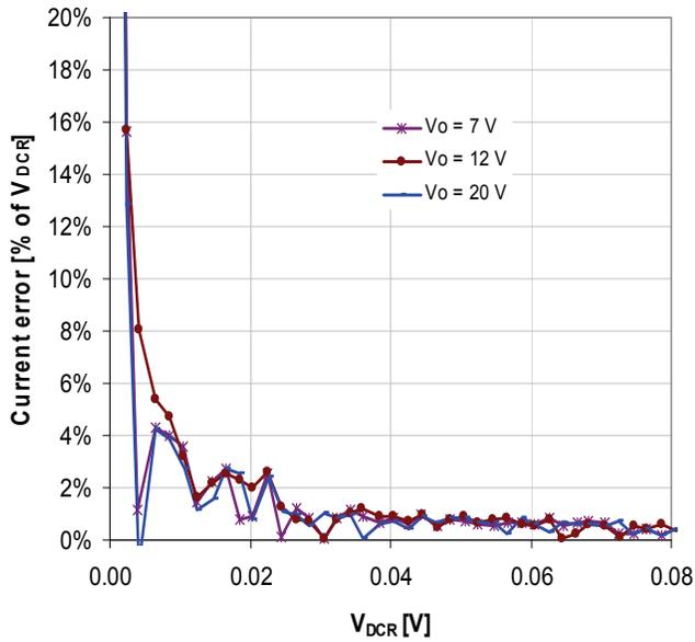
IR3725 CurrentMode - Error [%] (25 mV  $V_{DCR}$  full scale)
