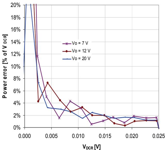
IR3725 PowerMode - Error [%] (9 mV  $V_{DCR}$  full scale)
