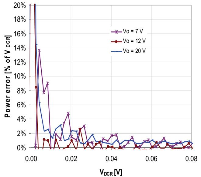
IR3725 PowerMode - Error [%] (25 mV  $V_{DCR}$  full scale)
