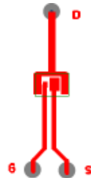
⑨ Mounted on minimum footprint full size board with metalized back and with small clip heatsink (still air)
